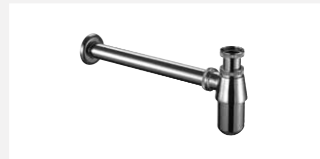
Classical basin bottle trap L: 367, W: 67, H: 197 Pipe length can be cut to size on site Code: W14
