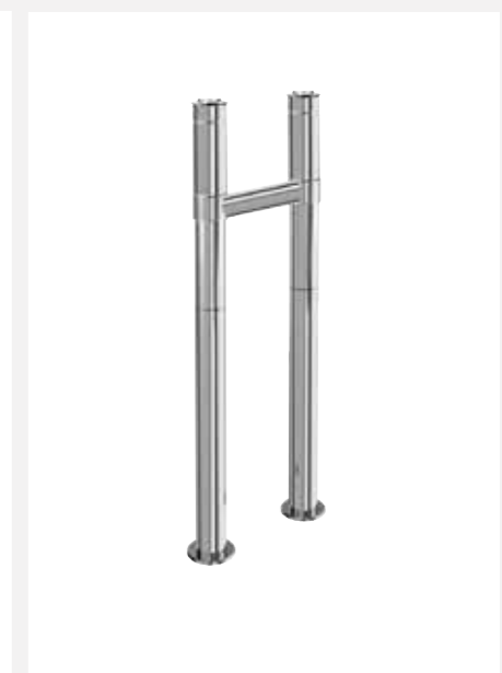
Stand pipes including horizontal support bar These are for use with baths where fittings are not rim or wall-mounted (Water runs through the pipes). Can be used with deck-mounted taps. D: 100, W: 280, H: 600 Code: W7
