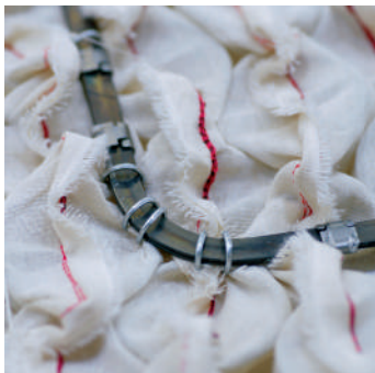
Hog rings on pocket-spring unit
