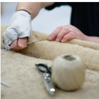
Stitching hair roll on No 2 box spring
